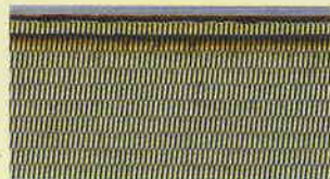
Appearance of edge joint welding of stainless steel wire mesh
