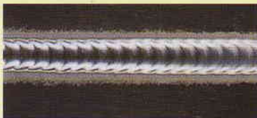
Bead Appearance in Rectangular Wave AC Pulsed TIG Welding of Aluminum
