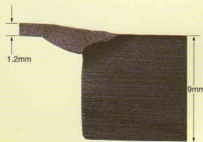
Macrostructure of joints welding section different in plate thickness
