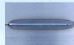
·Welding electric current:300A ·Welding voltage:22V ·Sheet thickness:3.2mm ·Wire diameter:φ1.2mm ·Welding speed:150cm/min ·Wire feeding speed:11.0m/min ·Protrusion:15mm
