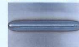
·Welding electric current:300A ·Welding voltage:22V ·Sheet thickness:3.2mm ·Wire diameter:φ1.2mm ·Welding speed:150cm/min ·Wire feeding speed:11.0m/min ·Protrusion:15mm
