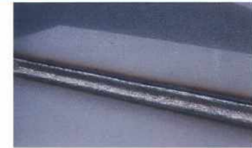
·Welding electric current:145A ·Welding voltage:23V ·Sheet thickness:2.0mm ·Wire diameter:φ1.2mm ·Welding speed:100cm/min
