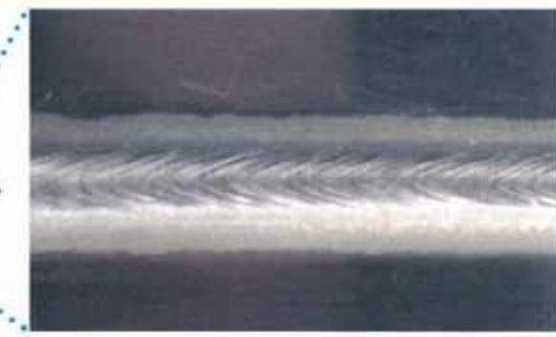
·Welding electric current:280A ·Welding voltage:21V ·Sheet thickness:1.5mm ·Wire diameter:φ1.2mm ·Welding speed:180cm/min
